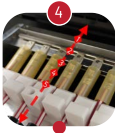
Up to 5 different programmable shrinking positions with independent process parameters
