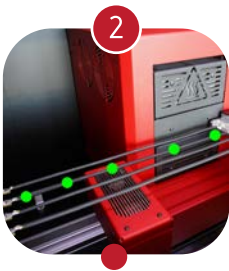
5 different shrinking positions with possibility of having different process parameters
