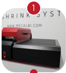
Optional side transporter to help the routing of heavier assemblies during the shrinking process
