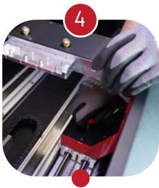
Adjustable product holders adaptable to different lengths and configurations of product
